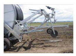
After retraction of the PE-pipe the machine supports can be carefully withdrawn with the tractor's hydraulic system. In doing so the cart is lifted into the transport position automatically.
