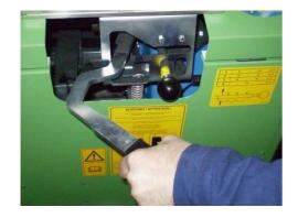
... and slacken the PE-pipe by carefully pressing the shut-off lever downward.
