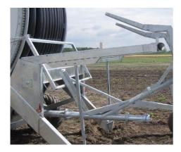
Unattended operation of the RAINSTAR is made possible by a final and safety shut-off. The final shut-off is actuated when the sprinkler cart pushes against the shut-off frame, which in turn operates the shut-off lever through a system of rods. This way the drive is stopped.
