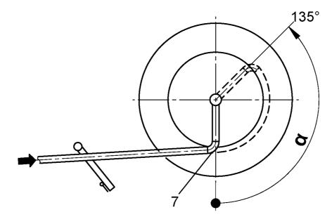
**Step 1:**Pull off the PE pipe and adjust the connecting bend (7) According to the table set up.
