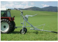
For easier PE-pipe pull-off the carts are equipped with a double draw-out hook. You pick up this hook with the tractor's toolbar and pull off the PE pipe.
