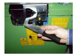
Pull the shut-off lever into the shut-off position....
