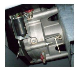
Open the drain valve on turbine
