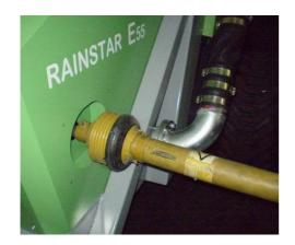
If required, you can rewind the PE-pipe also with the tractors PTO system
