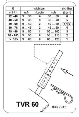
If discharge or retraction speed change substantially, the limiting bolt must be readjusted.
