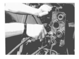
Couple the two hydraulic hoses with the hydraulic system of the tractor.
