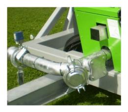
With an overpressure shut-off valve, the water supply to the machine is interrupted completely at the end of the irrigation run. When the valve closes, pressure rises in the supply line.
