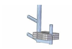
Place the appropriate number of balancing weights on the balancing pendulum of the cart.
