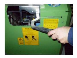
When the full operating pressure has been reached and clear water is discharged at the sprinkler's nozzle in a full jet without air bubbles, push the gear shift lever to the "PE-pipe retraction" position.
