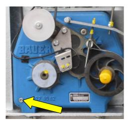
Drain screw for gear oil.
