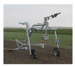
The high construction of both symmetric and asymmetric wheel carts provides maximum crop protection (Asymmetric wheel cart OPTIONAL). With infinitely variable track width the carts adapt to any crop row spacing. The width is symmetrically adjusted with the frame support member.
