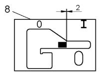
The shut-off point is reached when the PTO shaft no longer rotates. Adjust the shifting gate (8) in this position according to the drawing (2 mm / 0,08 inch)!
