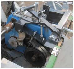
BAUER change-speed gearbox reduces the turbine speed according to the set turbine revs. The gearbox incorporates four gears. Reel drive stop at the end of the irrigation strip is ensured by disengagement of the tooth clutch.
