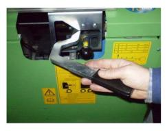
2. Pull the shut-off lever into the shut-off position and push it downward slowly and carefully...
