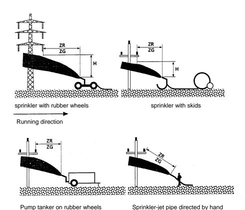
Attention: Do not spray slurry on insulators and masts!
