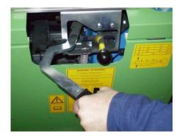
Slacken the PE-pipe by pushing down the gear shift lever carefully.
